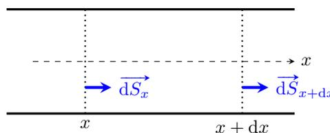
$$D_{m,x} = \rho v(x, t) S \quad \text{et} \quad D_{m,x+dx} = \rho v(x + dx, t) S.$$
